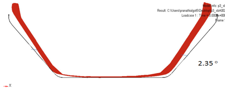
Figure 4.5: Springback angle 2.35° for sheet thickness of 0.3 mm.
